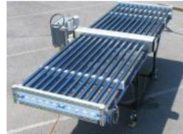
Figure 4. A solar/thermal array can be used to recharge the liquid desiccant—saving as much as 80% of the total electrical energy of conventional air conditioning.
